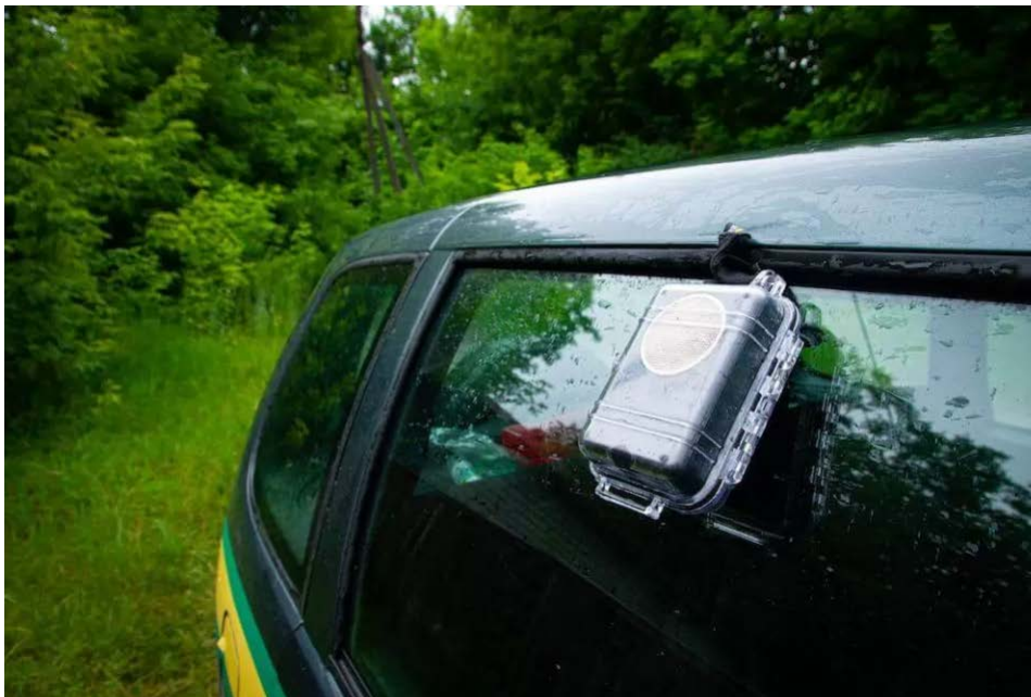
A bGeigie mounted on a 4WD vehicle of Chernobyl Radiation and Ecological Biosphere Reserve inside the Chernobyl Exclusion Zone.
